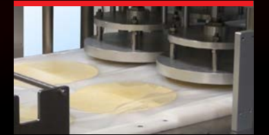
▲ B. Through a sensor, rested dough balls will be delivered to the pressing location to be pressed into finished products and be stacked at a set quantity, then delivered out by conveyor.
