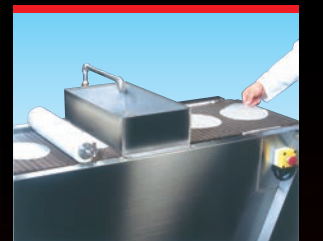
▲ 1. Set rice paper (manual) spray water. absorb excess water.
