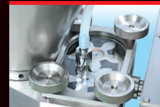
▲ Stuffing is extruded smoothly by a rotor pump.
